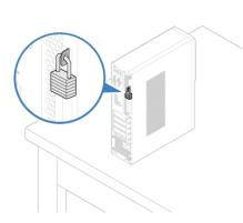
Locking the computer cover helps prevent unauthorized access to the inside of your computer. Your computer features a padlock loop so that the computer cover cannot be removed when a padlock is installed.
